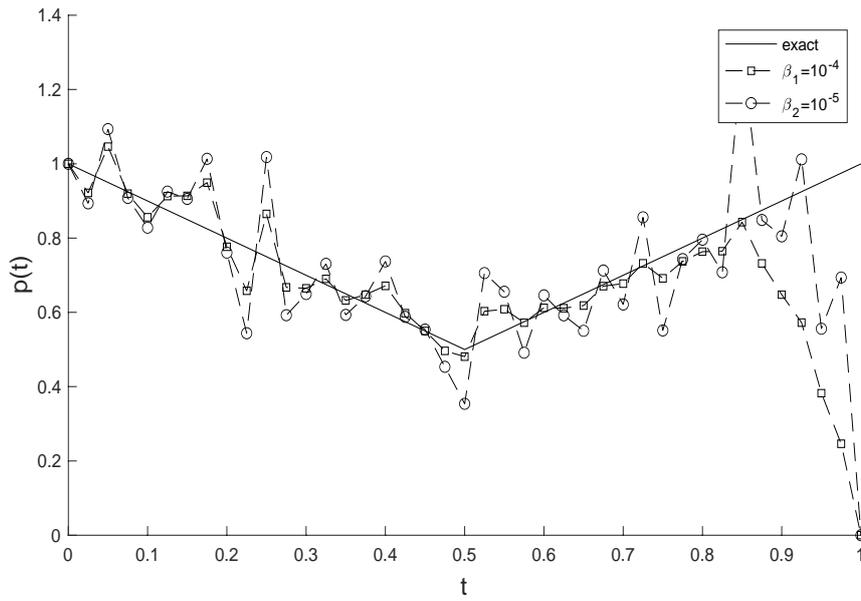
**Figure 14:** Numerical reconstructions and exact solution for  $p(t)$ , with regularization parameter  $\beta = \{10^{-5}, 10^{-4}\}$  and  $q = 0.1\%$  noise.
