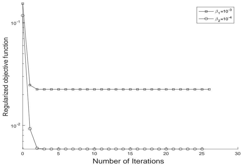
**Figure 17:** The regularized objective function (18), with regularization parameter  $\beta = \{10^{-4}, 10^{-3}\}$  and  $q = 1\%$  noise.
