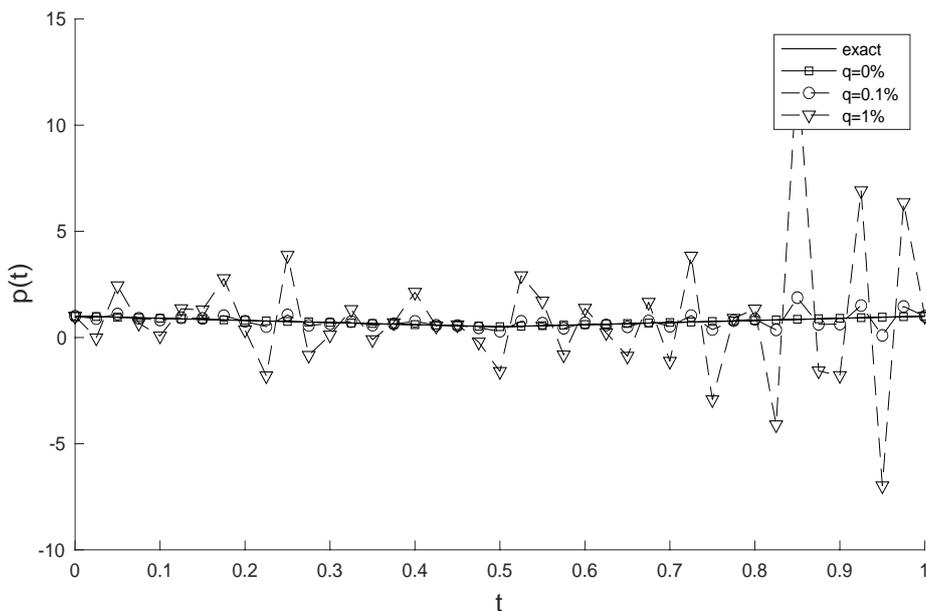
**Figure 12:** Numerical reconstructions in comparison with exact solution for  $p(t)$ , with noise level  $q = \{0, 0.1\%, 1\%\}$ , without regularization applied Example 2.
