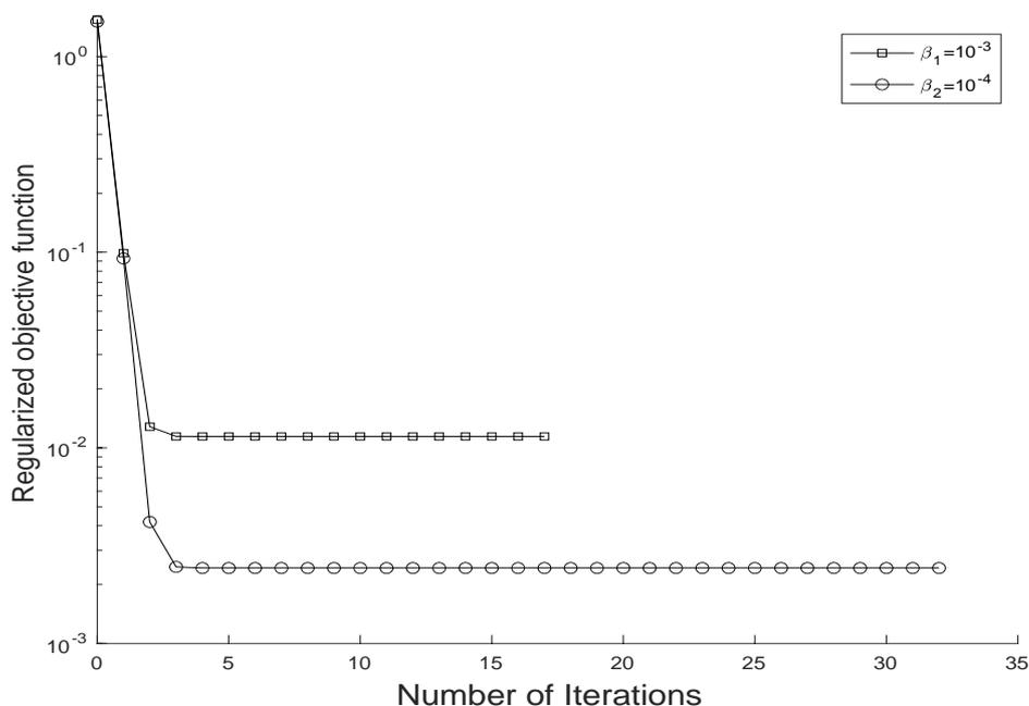
**Figure 7:** The regularized objective function (18), with regularization parameter  $\beta = \{10^{-4}, 10^{-3}\}$  and  $q = 1\%$  noise.
