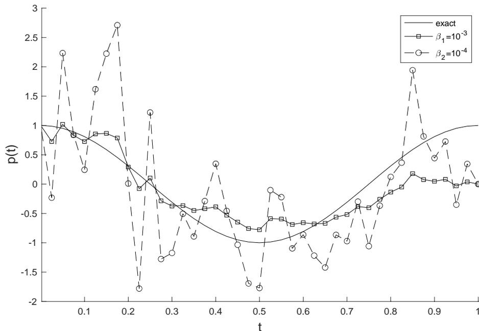
**Figure 8:** Numerical reconstructions and exact solution for  $p(t)$ , with regularization parameter  $\beta = \{10^{-4}, 10^{-3}\}$  and  $q = 5\%$  noise.
