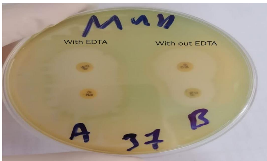
Figure 5: EDTA combined disc test
