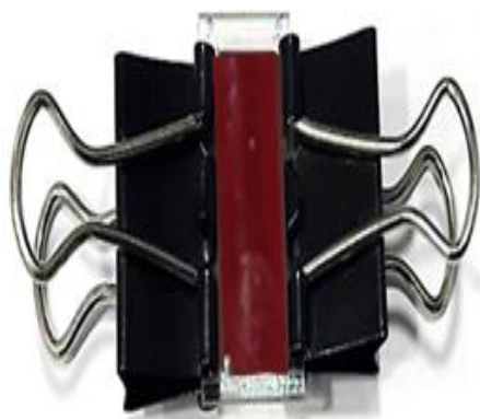
Figure 5: A picture of the prepared dye-sensitized solar cell.
