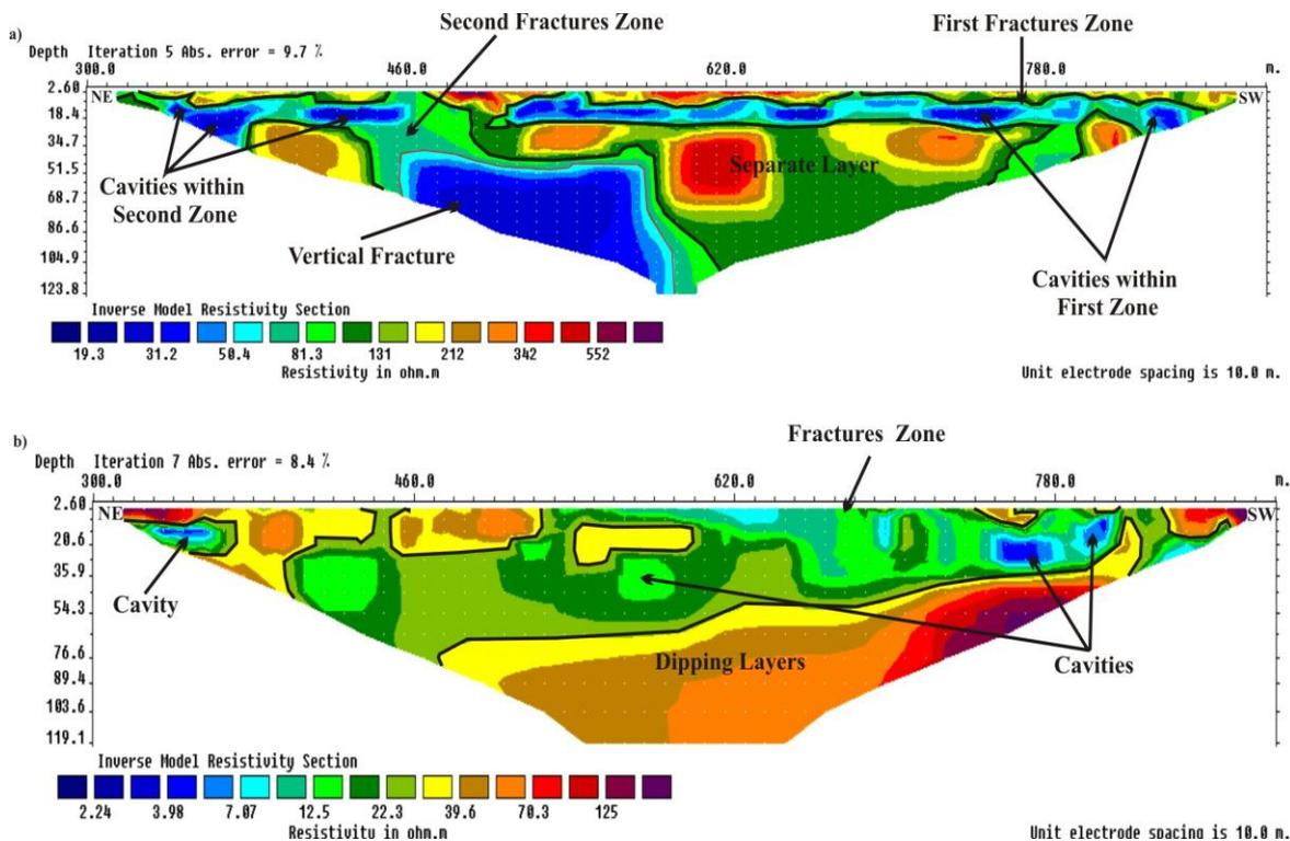
**Figure 6-** Shows the resistivity values of fracture zones within and out Abu- Jir fault zone, a) increasing resistivity values in inverse model of 2D imaging line (6), b) decreasing resistivity values in inverse model of 2D imaging line (10).
