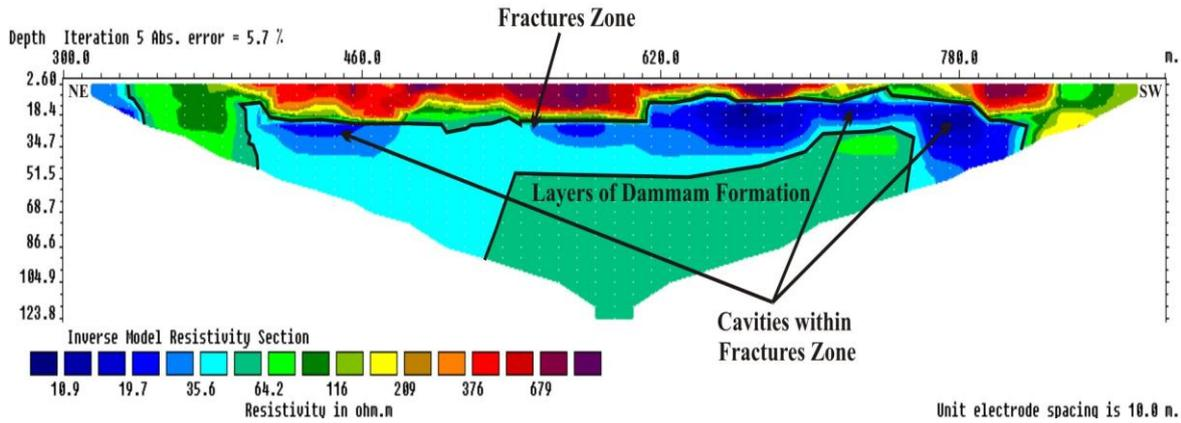
**Figure 4** - Shows the connection between the fractures zones to formed one fracture zone in inverse model of 2D imaging line (5).
