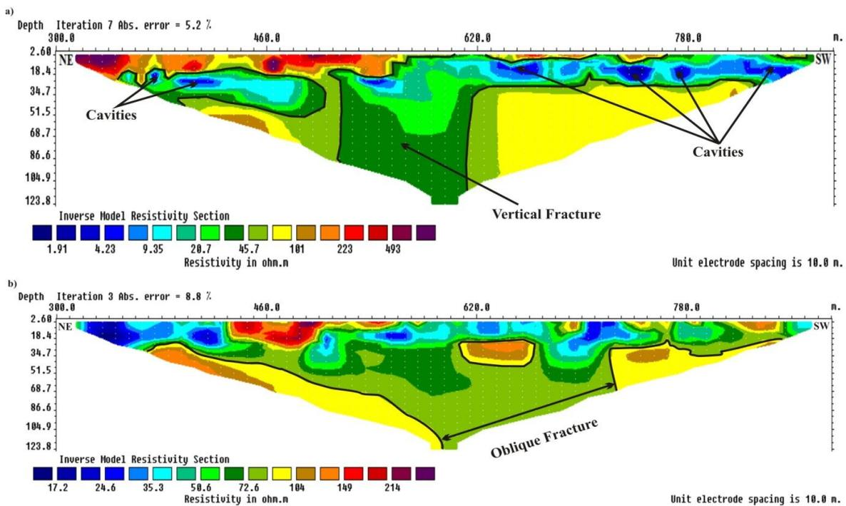
**Figure 5**- Shows the system types of fracture, a) vertical fracture in 2D imaging line (2), b) oblique fracture in 2D imaging line (3).
