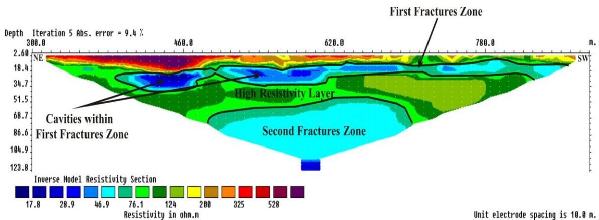
**Figure 3 -** Shows the types of fractures zones in inverse model of 2D imaging line (4).
