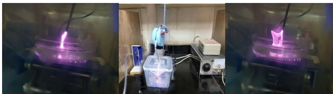
A (Atmospheric air only ) B (diagram of hybrid corona) C (mixing Argon gas with atmospheric air)
