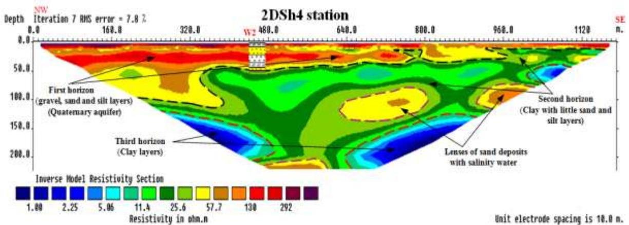
Figure 6- Shows the inverse model resistivity section for 2DSh4 station.
