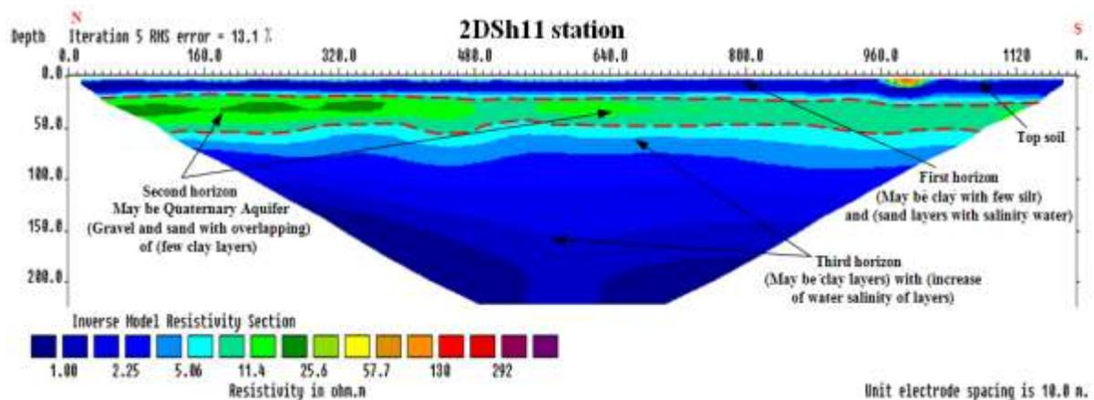
Figure 13 - Shows the inverse model resistivity section for 2DSh11 station.
