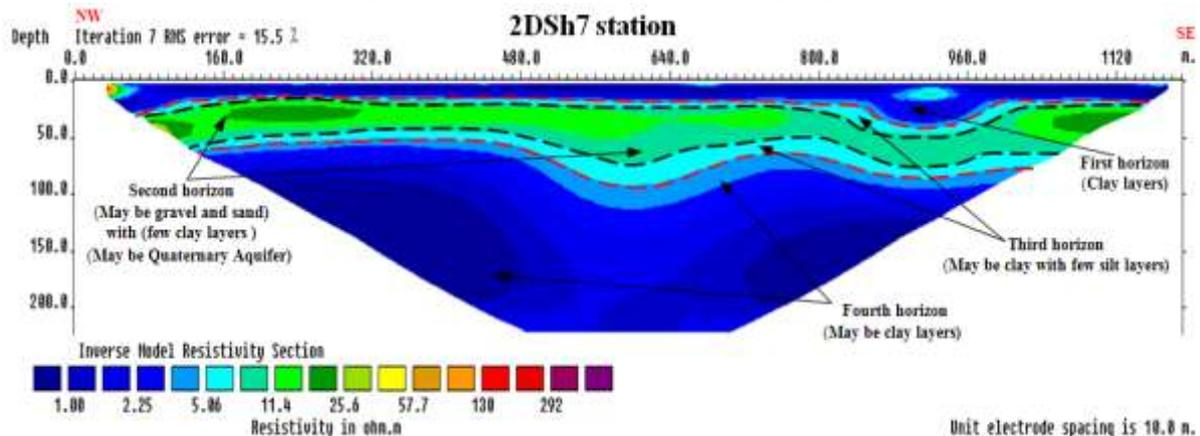
Figure 9 - Shows the inverse model resistivity section for 2DSh7 station.
