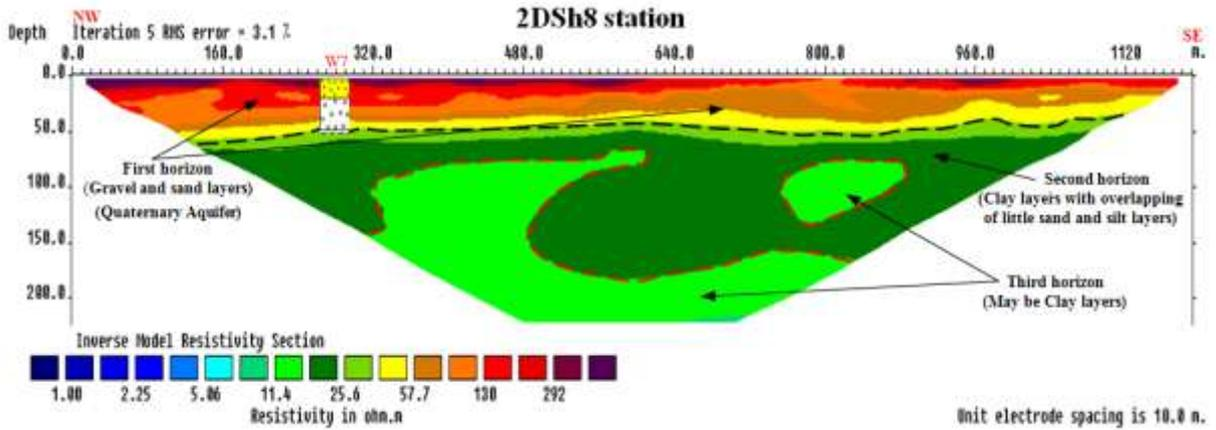
Figure 10 - Shows the inverse model resistivity section for 2DSh8 station.
