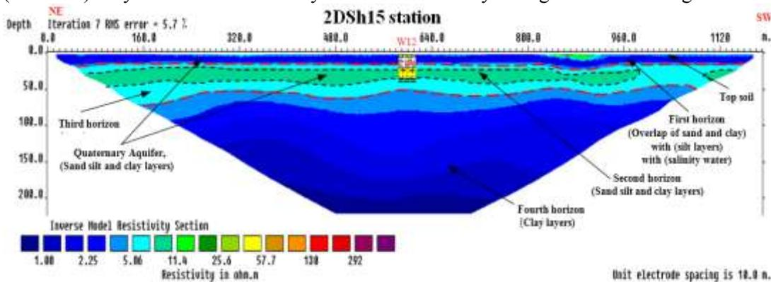
Figure 17 - Inverse model resistivity section for 2DSh15 station.
