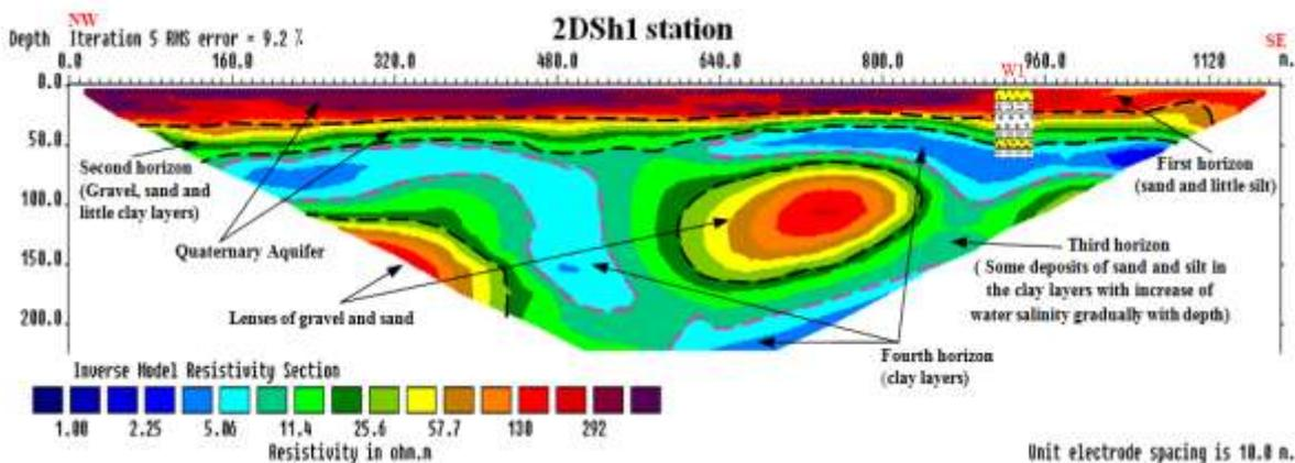
Figure 3 – Shows the inverse model resistivity section for 2DSh1 station.
