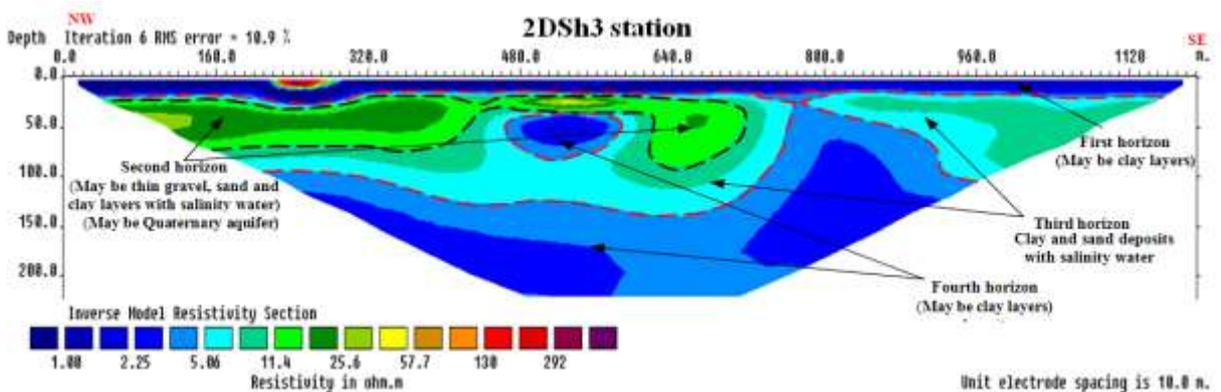
Figure 5- Shows the inverse model resistivity section for 2DSh3 station.
