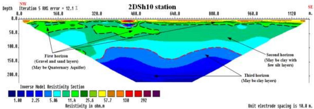
Figure 12 - Shows the inverse model resistivity section for 2DSh10 station.
