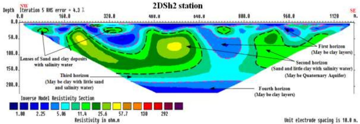
Figure 4 - Shows the inverse model resistivity section for 2DSh2 station.
