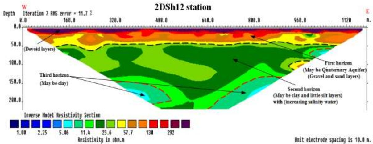
Figure 14 - Inverse model resistivity section for 2DSh12 station.
