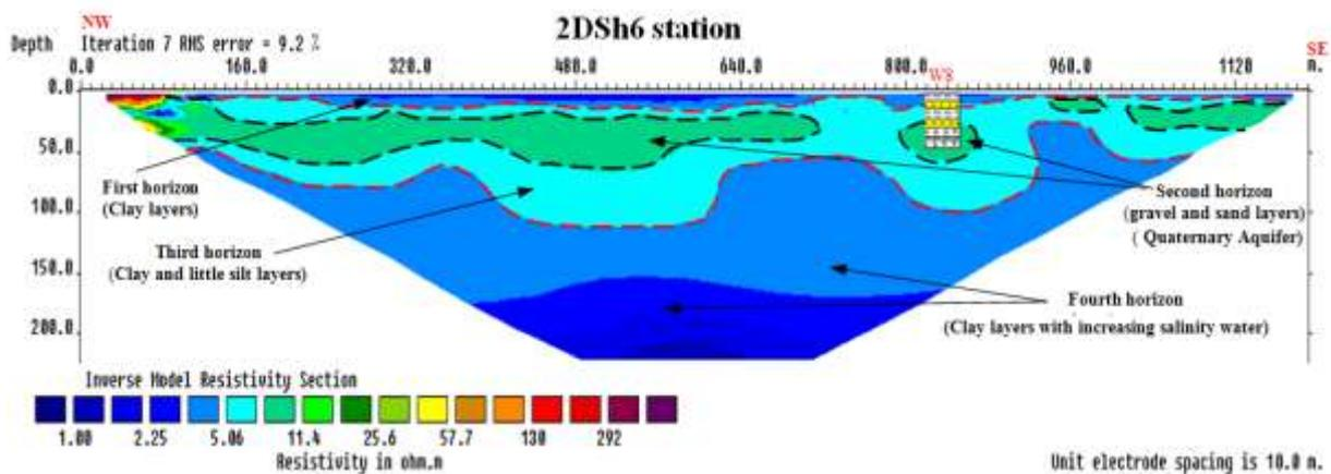
Figure 8 - Shows the inverse model resistivity section for 2DSh6 station.
