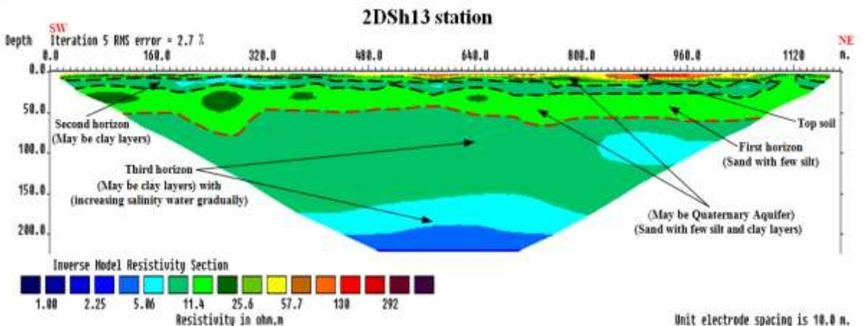
Figure 15 - Inverse model resistivity section for 2DSh13 station.
