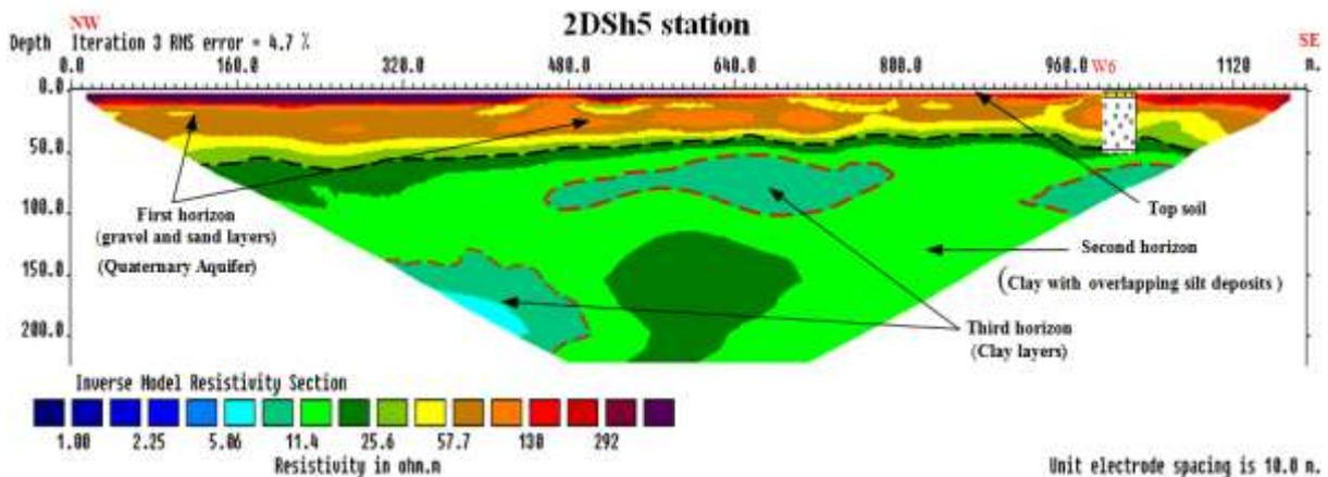
Figure 7 - Shows the inverse model resistivity section for 2DSh5 station.
