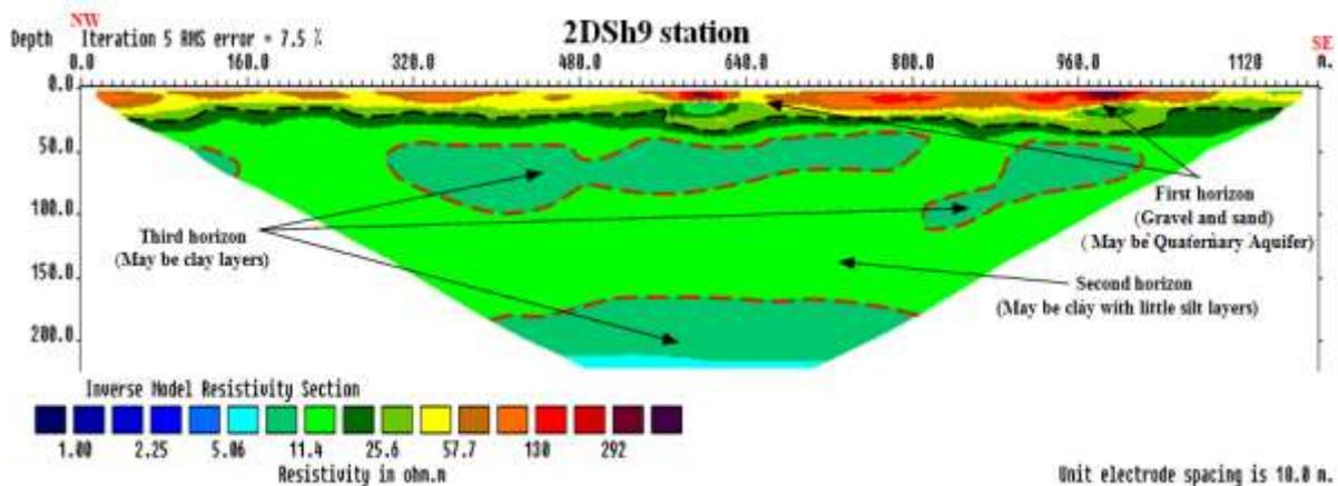
Figure 11- Shows the inverse model resistivity section for 2DSh9 station.
