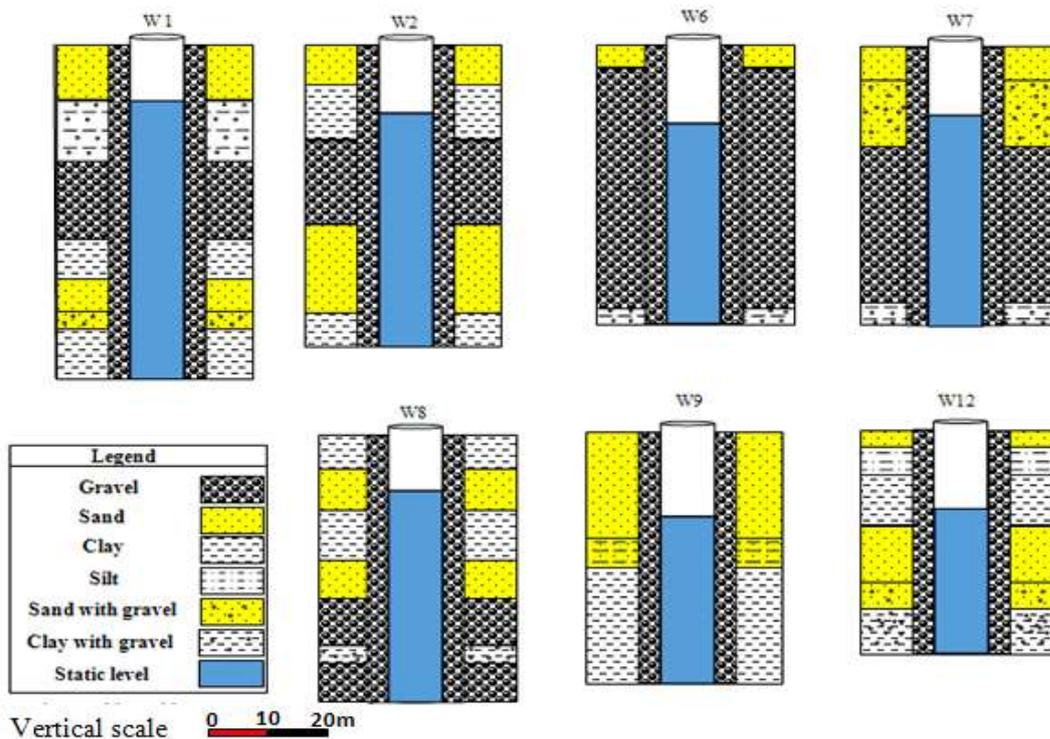
Figure 2 – Geological sections of the drilled wells in the study area [20].
