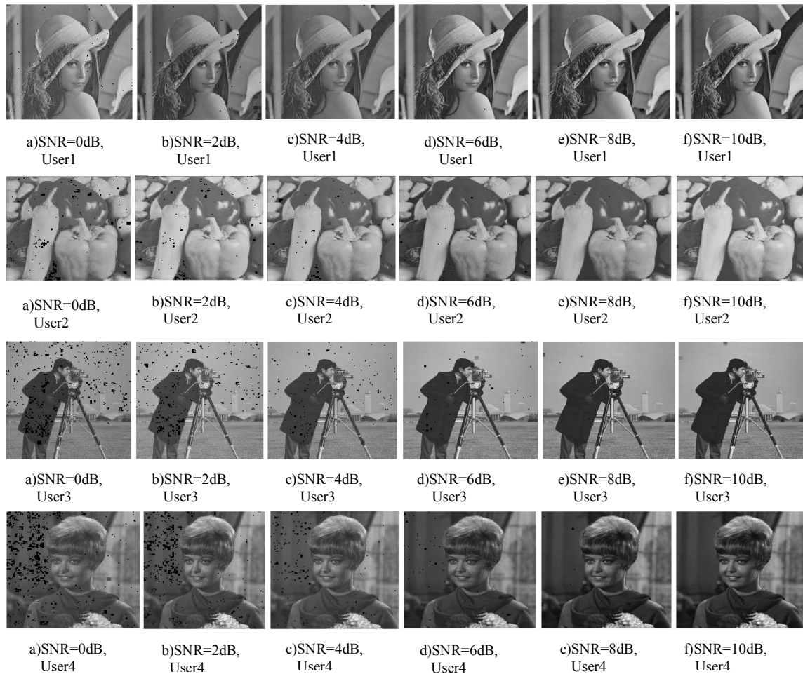
Figure 4- The received images of OFDM-IDMA system at different SNR values and for four different users without convolutional coding.
