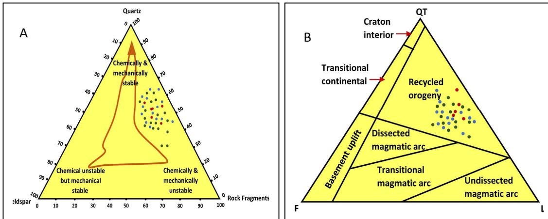
Figure 5- A: Ternary diagram of the stability of the sandstone of Injana Formation (based on Bjorlykke, 1983). B: plot of sandstone samples on the ternary diagram of Dickinson (1985).
