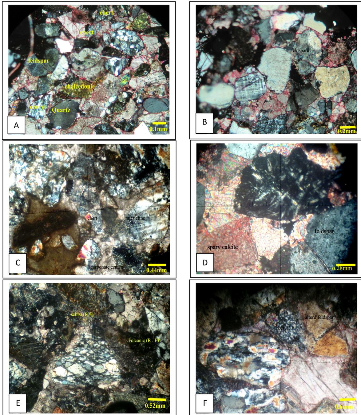
Figure- 2.(A) : Monocrystalline and polycrystalline with undulose extinction, ZW19, XPL.(B) : Feldspar orthoclase and microcline with cross hatching, ZK4, XPL. (C) : Carbonate skeletal rock fragment, ZW17, XPL. (D): Volcanic igneous rock fragment, A11, XPL. (E): Metamorphic rock fragment, A10, XPL. (F): Chert rock fragment (microcrystalline), ZW13, XPL.
