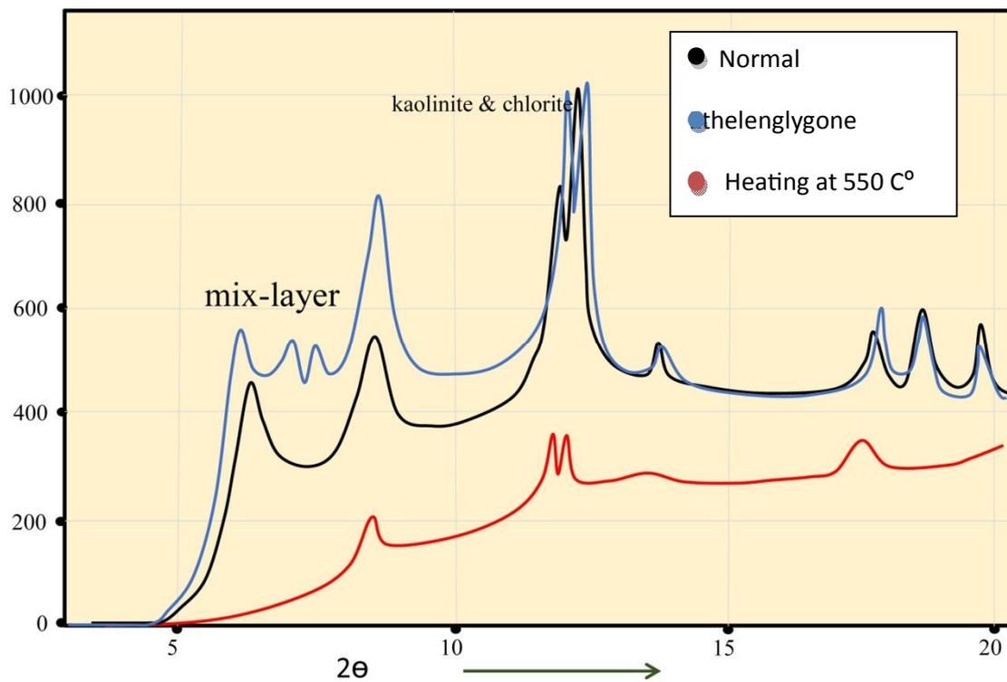
Figure 9- X-ray diffractograms for shows the clay mineral components in the sample ZW3 from Zawita section.
