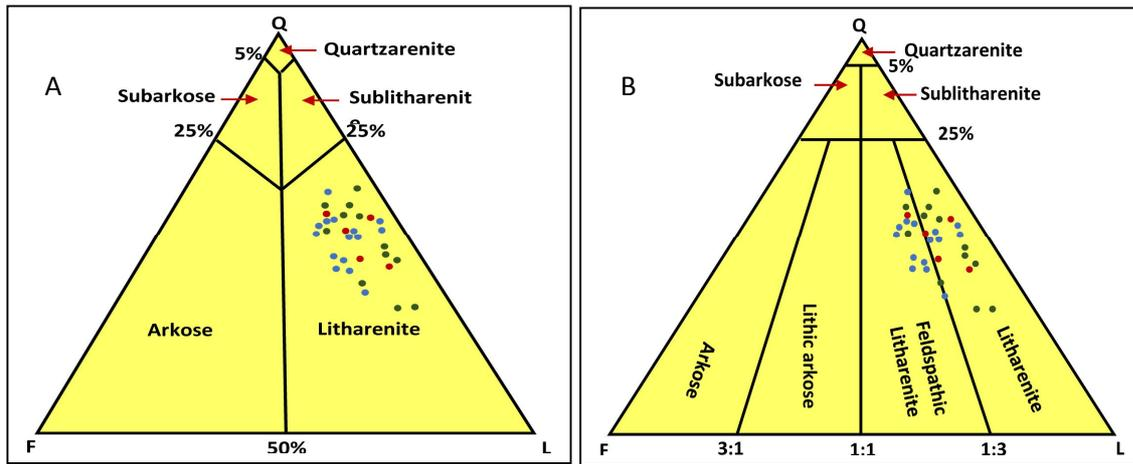
Figure 3- A Plot of sandstone samples on the ternary diagram of Pettijohn (1987), B classification of the sandstone of Injana Formation based on Folk (1974).
