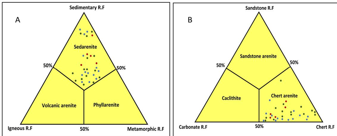
Figure 4- A Plot of Injana sandstone on the ternary diagram reflecting terminologies based on types of rock fragments of Injana Formation (based on Folk, 1974), B The relative percentage of types of sedimentary rock fragments based on Folk (1974).
