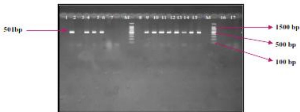
Figure 2 -Agarose gel electrophoresis for PCR product for detected bla OXA51like gene. Electrophoresis was performed on 2 % agarose gel and run with a 5volt/cm for 1.30 hr. stained with Ethidium Bromide and visualized on a UV transilluminator documentation system.M: 100bp ladder. Line 16 :( control negative, PCR reaction without DNA).Line 17 :( control negative, sensitive isolate). Line (1-15) meaning Ab1-Ab15.
